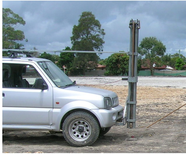
Figure 3. The weight dropping system
