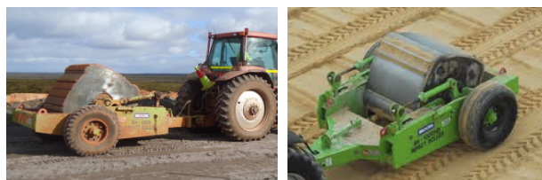
Figure 1. An example of RDC – Broons BH-1300 4-sided impact roller.
