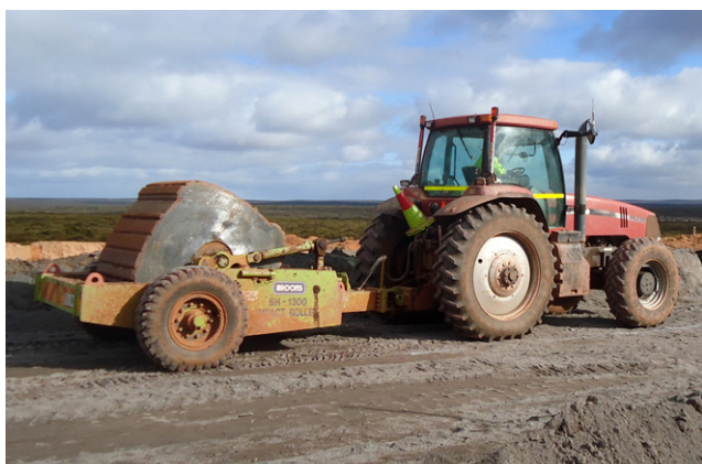
Figure 1. 8 t four-sided impact roller
