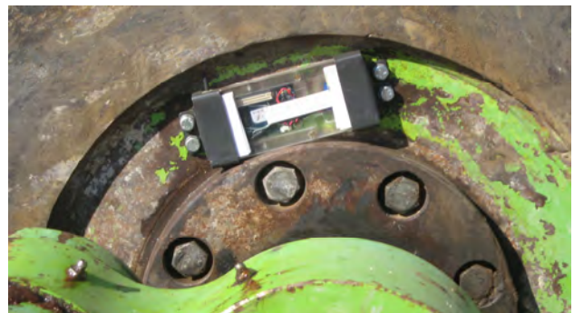
Figure 3. Transmitter and accelerometer device mounted directly onto impact module.
