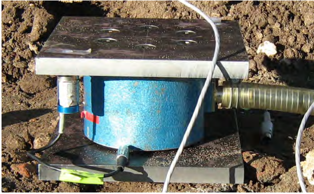
Figure 4. Load cell with accelerometers prior to embedment in the ground.
