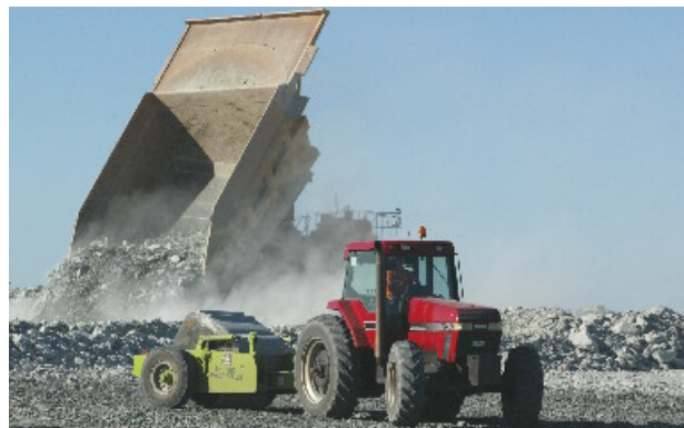
Figure 11: The impact roller and a dump truck on a mine waste tip.
