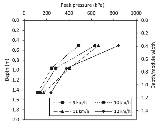
**Fig. 4.** Measured peak pressure increasing with towing speed.
