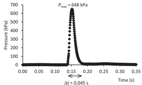
**Fig. 3.** Measured impulse pressure at 0.5 m depth.
