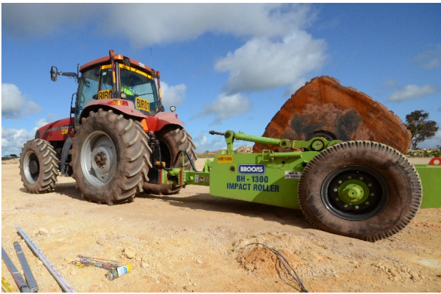
Figure 1. Broons 4-sided, 8-tonne, BH-1300 impact roller.
