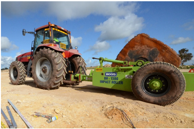
Figure 1. Broons 4-sided, 8-tonne, BH-1300 impact roller.
