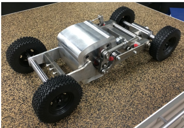
Figure 3. Model of Broons BH-1300, 4-sided impact roller. (The dual spring-linkages can be seen on the left- and right-hand sides of the module.)
