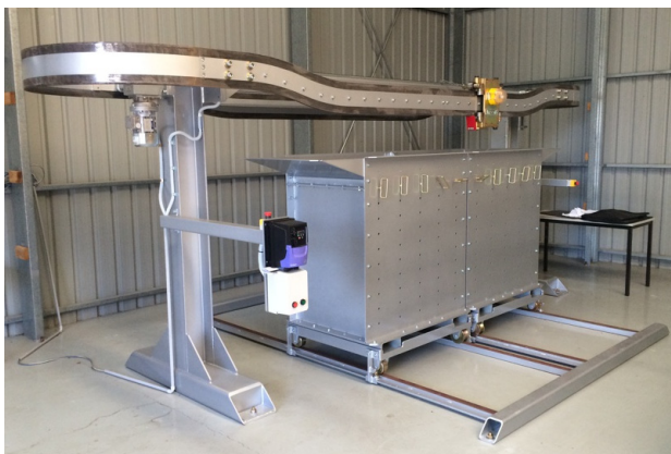
Figure 2. Test rig for scale model impact roller.
