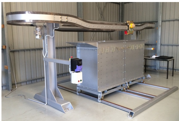
Figure 2. Test rig for scale model impact roller.
