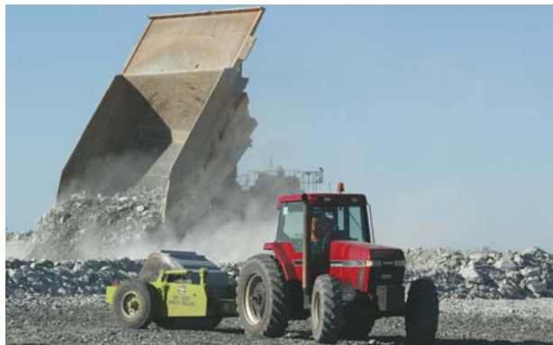
Figure 4: The impact roller and a dump truck on a mine waste tip.
