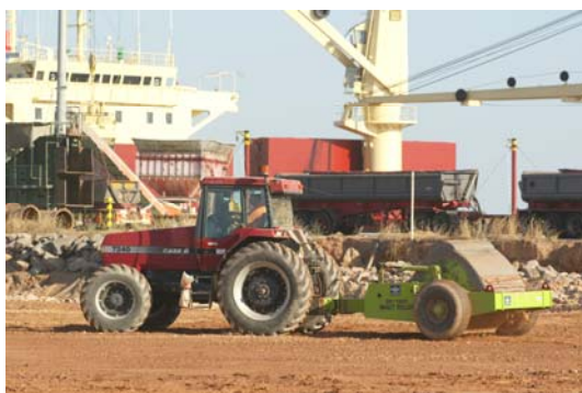
Figure 1: The “square” impact roller.
