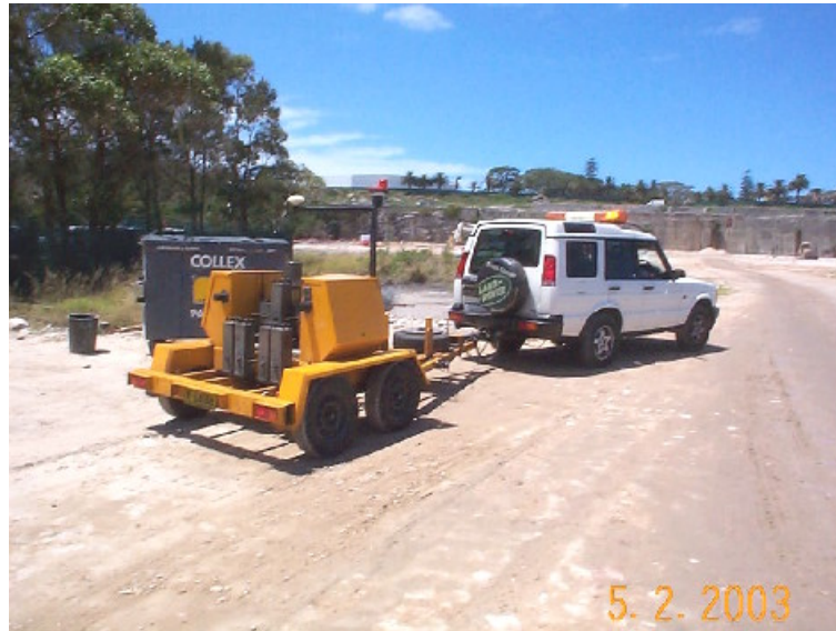
Figure 2: HFWD Test Rig at Bunnerong Site.
