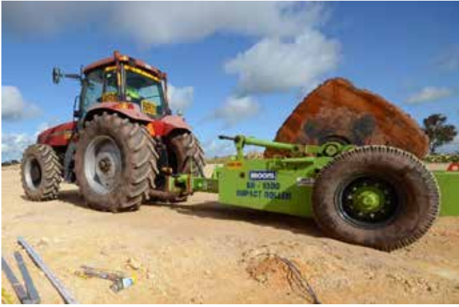
Figure 1. Broons BH-1300 4-sided impact roller used in compaction trial.
