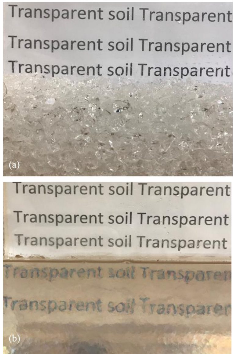
Figure 2.2: Transparent soil with text viewed from behind a 60 mm thickness of fused quartz with: (a) no pore fluid, (b) STSI pore fluid.
