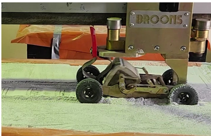
Figure 21: First pass of 1:13 RDC model on loose, dry MAB-1 simulant.
