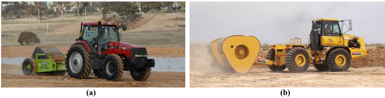
Figure 4: Rolling dynamic compaction modules: (a) 4-sided (Broons); and (b) 3-sided (Landpac).
