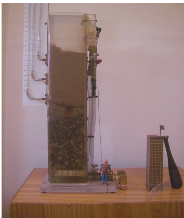
Figure 28: Liquefaction sand column.
