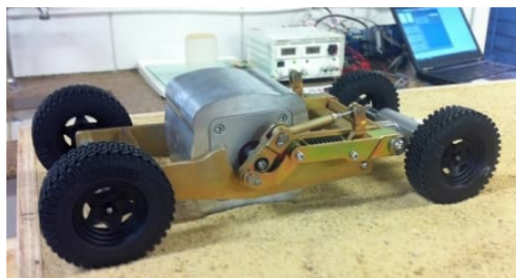
Figure 9: Scale model (1:13) replica of Broons BH-1300 4-sided impact roller.
