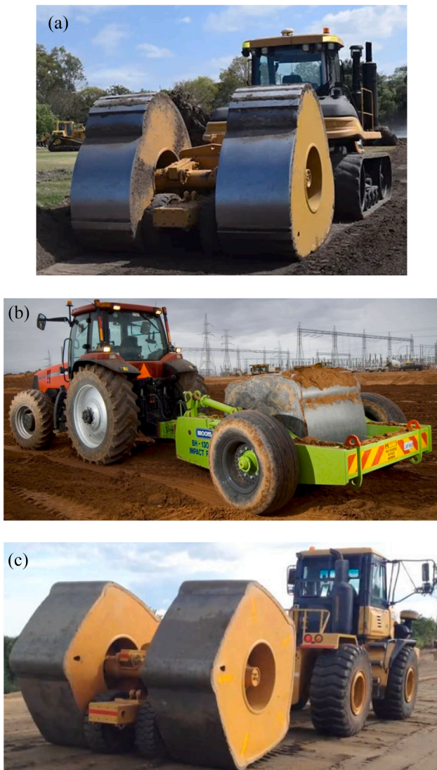
Fig. 1. Different module designs: (a) 3-sided (Landpac), (b) 4-sided (Broons), (c) 5-sided (Landpac).
