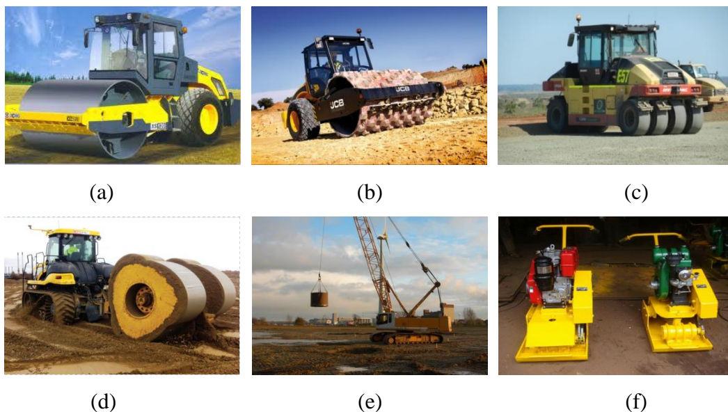
Figure 2.1 Various ground compaction methods: (a) drum rollers; (b) pad foot rollers; (c) pneumatic multi-tyre rollers; (d) rolling dynamic compaction; (e) heavy tamping; and (f) vibrating plates.
