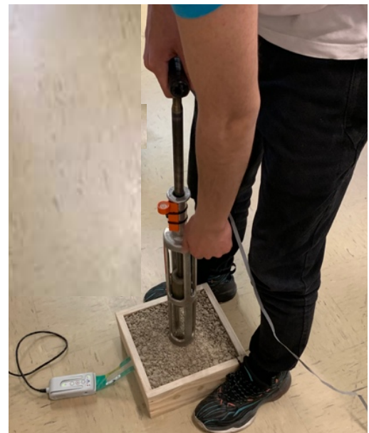
Fig. 11: Sensor calibration using an instrumented Proctor compaction hammer.
