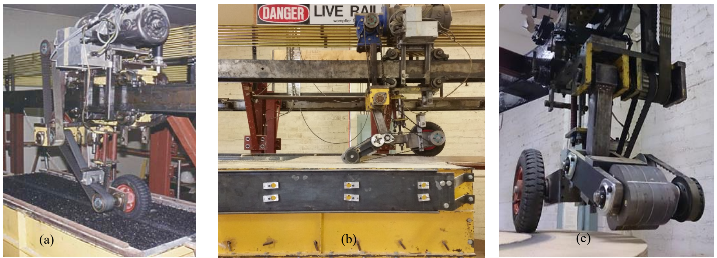
Fig. 5: University of Sydney test apparatus: (a) original pavement facility, (b) modified facility for RDC testing, (c) details of 1:20 scale model.
