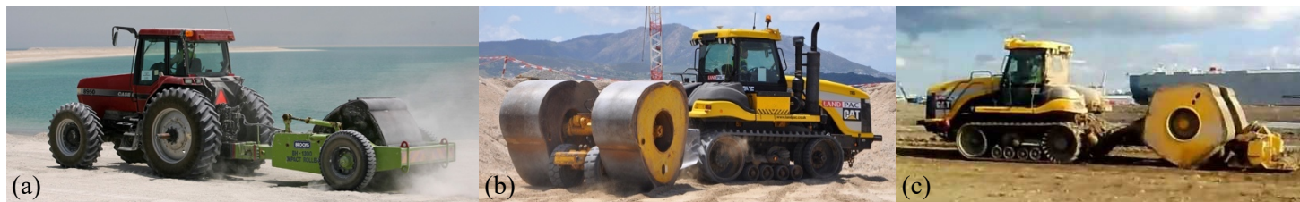
Fig. 1: Rolling dynamic compaction modules: (a) 4-sided (Broons); (b) 3-sided (Landpac); (c) 5-sided (Landpac).
