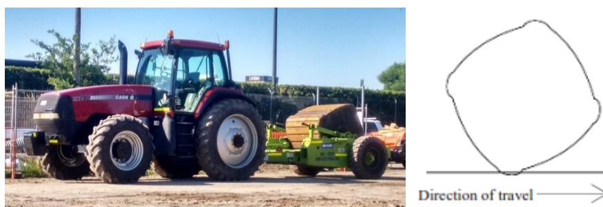
Figure 1: Dynamic rolling module towed in a frame by a 4-wheel drive tractor and cross section of a four-sided HEIC module (Bierbaum et al. , 2010)
