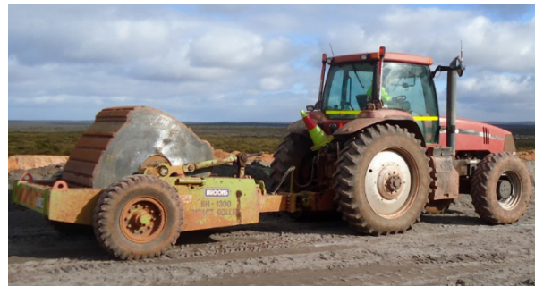
Figure 1. 4-sided impact roller.
