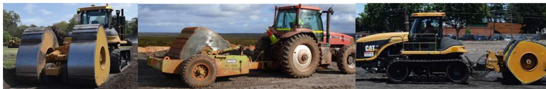
Fig. 2 From left to right, examples of 3-, 4- and 5-sided impact rollers. (Photos 1 and 3 from Landpac [5]. Photo 2 from broonsimpactrollers.com .)
